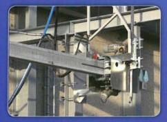
The straight vertical stroke of its probe provides precision and a high force of penetration.
